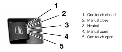
Toll operation (one-touch) takes place in the closing or opening direction immediately after the switch position "one touch closed" or "one-touch open" has been reached. The power windows are activated in the initial closed/open lock-in positions as long as the button is held in this position. Anti-trapping protection is active in both one-touch and manual operation.
